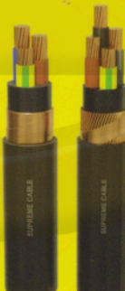
NYSY, NYCY SNI IEC 60502-1, IEC 60502-1 0.6/1(1.2) kV Multicore, power & control cable, copper conductor, PVC insulated, copper wire or copper tape screened, PVC sheathed. Main used for street and outdoor lighting, house services in urban network, indoor, in ducts installation or in the open where not sustain mechanical damage.
