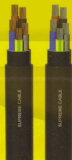
NYY, NAYY SNI IEC 60502-1 0.6/1(1.2) kV Single, multicore, power & control cable, copper or aluminium conductor, PVC insulated, PVC sheathed. Main used for indoor, in duct installation or for laying in the ground where not sustain mechanical damage.
