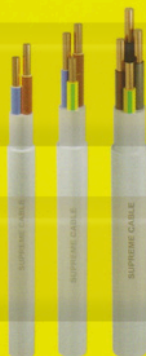
NYM SNI 04-6629.4, IEC 60227-4 300/500 Volts Multicores, copper conductor, PVC insulated, PVC sheathed, round or flat type. Main used for permanent installation in conduit under plaster or exposed installation in dry location.
