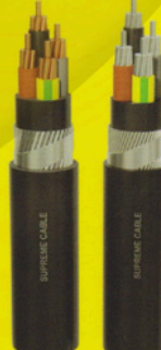
NYFGbY, NYRGbY, NAYFGbY, NAYRGbY SNI IEC 60502-1 0.6/1(1.2) kV Multicores, power & control cable, copper or aluminium conductor, PVC insulated, round steel wire or steel tape armoured, PVC sheathed. Main used for indoor and outdoor installation direct burial, preferably used where mechanical stress must be envisaged.
